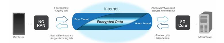
When traveling through an IPsec tunnel, user plane traffic (that is, traffic from the user's device) or control plane traffic (that is, information from the network's control interface) cannot be captured, modified, or injected by an unauthorized entity.
